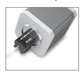
The BF-820 Bare Fiber Holder completely encircles the fiber, probibiting ambient light from interfering with power measurements.
